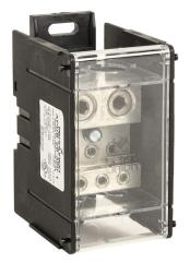
Penn-Union open power distribution block, finger-safe, 620A, 1-pole, line side: 2 openings accept 350 MCM to 6 AWG Cu/AL, load side: 6 openings accept 2/0 AWG to 14 AWG Cu/AL, DIN rail or panel mount, UL 1953 listed.
