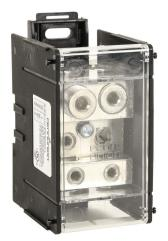
Penn-Union open power distribution block, finger-safe, 760A, 1-pole, line side: 2 openings accept 500 MCM to 4 AWG Cu/AL, load side: 4 openings accept 4/0 AWG to 6 AWG Cu/AL, DIN rail or panel mount, UL 1953 listed.
