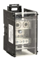
Penn-Union open power distribution block, finger-safe, 760A, 1-pole, line side: 2 openings accept 500 MCM to 4 AWG Cu/AL, load side: 12 openings accept 4 AWG to 14 AWG Cu/AL, DIN rail or panel mount, UL 1953 listed.
