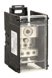
Penn-Union open power distribution block, finger-safe, 380A, 1-pole, line side: 1 openings accept 500 MCM to 4 AWG Cu/AL, load side: 6 openings accept 2/0 AWG to 14 AWG Cu/AL, DIN rail or panel mount, UL 1953 listed.
