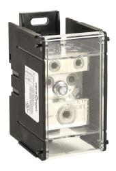
Penn-Union open power distribution block, finger-safe, 380A, 1-pole, line side: 1 openings accept 500 MCM to 4 AWG Cu/AL, load side: 4 openings accept 4/0 AWG to 6 AWG Cu/AL, DIN rail or panel mount, UL 1953 listed.
