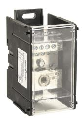
Penn-Union open power distribution block, finger-safe, 310A, 1-pole, line side: 1 openings accept 350 MCM to 6 AWG Cu/AL, load side: 12 openings accept 4 AWG to 14 AWG Cu/AL, DIN rail or panel mount, UL 1953 listed.
