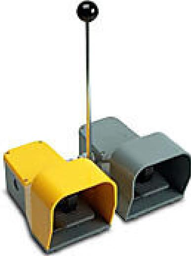
AutomationDirect electric foot switch, double, ABS plastic foot guard(s), (1) yellow and (1) gray, momentary, (1) N.O. and (1) N.C. snap action contact per switch, ABS plastic operator, safety anti-trip pedal, gray, ABS plastic base.
