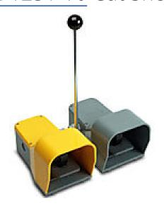
AutomationDirect electric foot switch, double, ABS plastic foot guard(s), (1) yellow and (1) gray, momentary, (1) N.O. and (1) N.C. snap action contact per switch, ABS plastic operator, safety antitrip pedal, gray, ABS plastic base.
