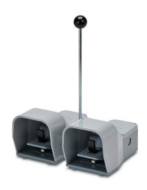
AutomationDirect electric foot switch, double, die-cast aluminum foot guard(s), (2) gray, momentary, (2) N.O. and (2) N.C. slow action contacts per switch, ABS plastic operator, safety anti-trip pedal, gray, ABS plastic base.
