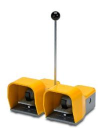
AutomationDirect electric foot switch, double, die-cast aluminum foot guard(s), (2) yellow, momentary, (2) N.O. and (2) N.C. snap action contacts per switch, ABS plastic operator, safety anti-trip pedal, gray, ABS plastic base.
