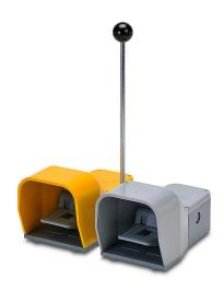
AutomationDirect electric foot switch, double, die-cast aluminum foot guard(s), (1) yellow and (1) gray, momentary, (2) N.O. and (2) N.C. slow action contacts per switch, ABS plastic operator, free moving pedal, gray, ABS plastic base.
