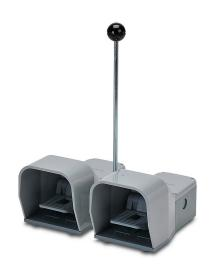
AutomationDirect electric foot switch, double, die-cast aluminum foot guard(s), (2) gray, momentary, (2) N.O. and (2) N.C. slow action contacts per switch, ABS plastic operator, free moving pedal, gray, ABS plastic base.
