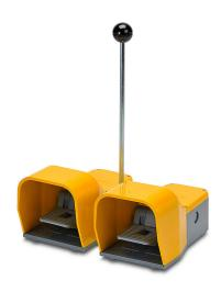
AutomationDirect electric foot switch, double, die-cast aluminum foot guard(s), (2) yellow, momentary, (2) N.O. and (2) N.C. slow action contacts per switch, ABS plastic operator, free moving pedal, gray, ABS plastic base.
