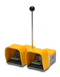
AutomationDirect electric foot switch, double, die-cast aluminum foot guard(s), (2) yellow, momentary, (2) N.O. and (2) N.C. snap action contacts per switch, ABS plastic operator, free moving pedal, gray, ABS plastic base.
