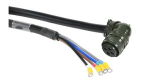
LS Electric power cable, mating connectors, 65.6ft/20m cable length. For use with LS Electric 230 VAC APM-FF55D series servo motors without brake.
