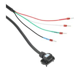
LS Electric power cable, mating connectors, 32.8ft/10m cable length. For use with 100W-1 kW LS Electric FBL/FCL series servo motors used with iX7 series drives.
