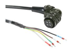
LS Electric power cable, mating connectors, 32.8ft/10m cable length. For use with LS Electric 230 VAC APM-FE15A servo motors without brake.
