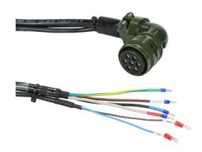
LS Electric power cable, mating connectors, 16.4ft/5m cable length. For use with LS Electric 230 VAC APM-FF35D servo motors with brake.
