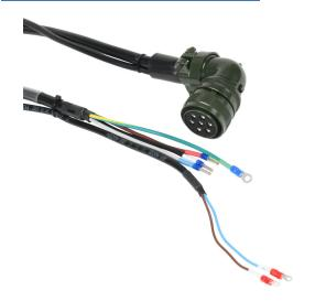
LS Electric power cable, mating connectors, 16.4ft/5m cable length. For use with LS Electric 230 VAC APM-FF35D and 460 VAC APM-FFP35D series servo motors with brake.
