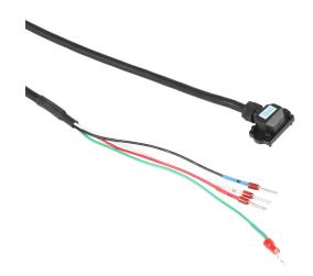
LS Electric power cable, mating connectors, 16.4ft/5m cable length. For use with 100W-1 kW LS Electric FBL/FCL series servo motors used with L7P series drives.
