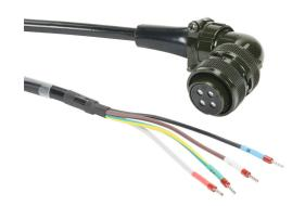
LS Electric power cable, mating connectors, 16.4ft/5m cable length. For use with LS Electric 230 VAC APM-FE15A servo motors without brake.
