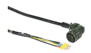
LS Electric power flex cable, mating connectors, 65.6ft/20m cable length. For use with LS Electric 460 VAC APM-FFP55D and APM-FFP75D series servo motors without brake.
