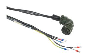
LS Electric power flex cable, mating connectors, 32.8ft/10m cable length. For use with LS Electric 230 VAC APM-FF35D and 460 VAC APM-FFP35D series servo motors with brake.
