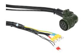
LS Electric power flex cable, mating connectors, 32.8ft/10m cable length. For use with LS Electric 460 VAC APM-FFP55D and APM-FFP75D series servo motors with brake.
