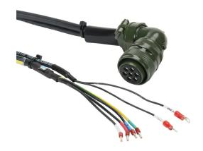
LS Electric power flex cable, mating connectors, 16.4ft/5m cable length. For use with LS Electric 230 VAC APM-FE15A servo motors with brake.
