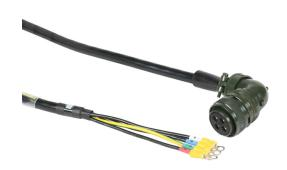
LS Electric power flex cable, mating connectors, 16.4ft/5m cable length. For use with LS Electric 460 VAC APM-FFP55D and APM-FFP75D series servo motors without brake.
