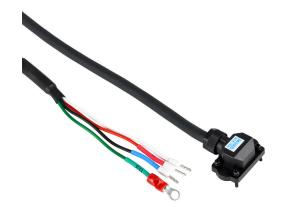
LS Electric power flex cable, mating connectors, 9.8ft/3m cable length. For use with 100W-1 kW LS Electric FBL/FCL series servo motors used with L7C series drives.
