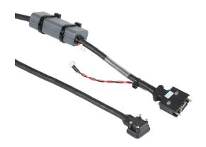
LS Electric encoder feedback flex cable, mating connectors, 32.8ft/10m cable length. For use with 100W-1 kW LS Electric FBL/ FCL series servo motors with 19-bit encoders. (1) AA ER6V lithium battery included.
