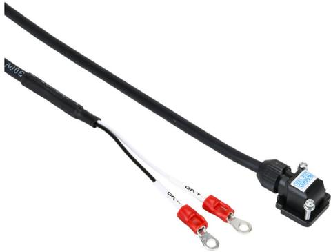
LS Electric brake cable, mating connectors, 16.4ft/5m cable length. For use with 100W-1 kW LS Electric FBL/FCL series servo motors with brake.
