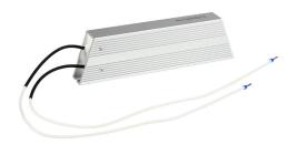
LS Electric braking resistor, 300W, 82 ohm, encapsulated. For use with LS Electric 460 VAC 1 kW drives.
