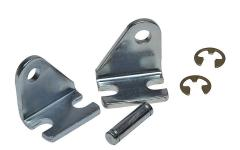
NITRA mounting bracket, pivot with pin, zinc plated steel. For use with 1-1/4in bore A-series cylinders.
