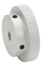
SureMotion timing pulley, aluminum, 0.08in MXL pitch, 80 tooth, 2.037in pitch diameter, 5/16in bore, hub without flanges. For use with 1/4in wide belt.
