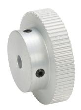
SureMotion timing pulley, aluminum, 0.08in MXL pitch, 72 tooth, 1.833in pitch diameter, 1/4in bore, hub without flanges. For use with 1/4in wide belt.
