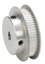
SureMotion timing pulley, aluminum, 0.08in MXL pitch, 60 tooth, 1.528in pitch diameter, 1/4in bore, hub with flanges. For use with 1/4in wide belt.
