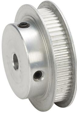
SureMotion timing pulley, aluminum, 0.08in MXL pitch, 60 tooth, 1.528in pitch diameter, 1/4in bore, hub with flanges. For use with 1/4in wide belt.
