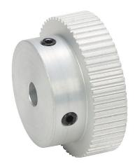
SureMotion timing pulley, aluminum, 0.08in MXL pitch, 60 tooth, 1.528in pitch diameter, 1/4in bore, hub without flanges. For use with 1/4in wide belt.
