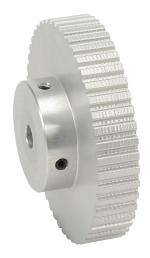
SureMotion timing pulley, aluminum, 1/5in XL pitch, 48 tooth, 3.056in pitch diameter, 5/16in bore, hub without flanges. For use with 3/8in wide belt.
