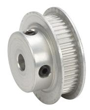
SureMotion timing pulley, aluminum, 0.08in MXL pitch, 48 tooth, 1.222in pitch diameter, 1/4in bore, hub with flanges. For use with 1/4in wide belt.
