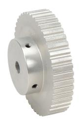
SureMotion timing pulley, aluminum, 1/5in XL pitch, 44 tooth, 2.801in pitch diameter, 5/16in bore, hub without flanges. For use with 3/8in wide belt.
