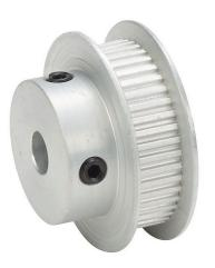
SureMotion timing pulley, aluminum, 0.08in MXL pitch, 44 tooth, 1.12in pitch diameter, 1/4in bore, hub with flanges. For use with 1/4in wide belt.
