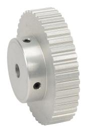
SureMotion timing pulley, aluminum, 1/5in XL pitch, 42 tooth, 2.674in pitch diameter, 5/16in bore, hub without flanges. For use with 3/8in wide belt.
