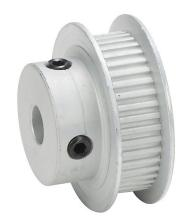
SureMotion timing pulley, aluminum, 0.08in MXL pitch, 42 tooth, 1.07in pitch diameter, 1/4in bore, hub with flanges. For use with 1/4in wide belt.
