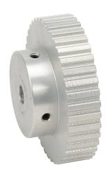
SureMotion timing pulley, aluminum, 1/5in XL pitch, 40 tooth, 2.546in pitch diameter, 5/16in bore, hub without flanges. For use with 3/8in wide belt.
