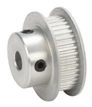
SureMotion timing pulley, aluminum, 0.08in MXL pitch, 40 tooth, 1.019in pitch diameter, 1/4in bore, hub with flanges. For use with 1/4in wide belt.
