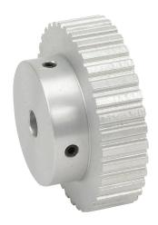
SureMotion timing pulley, aluminum, 1/5in XL pitch, 36 tooth, 2.292in pitch diameter, 5/16in bore, hub without flanges. For use with 3/8in wide belt.
