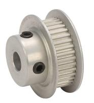
SureMotion timing pulley, aluminum, 0.08in MXL pitch, 36 tooth, 0.917in pitch diameter, 1/4in bore, hub with flanges. For use with 1/4in wide belt.
