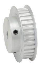
SureMotion timing pulley, aluminum, 1/5in XL pitch, 32 tooth, 2.037in pitch diameter, 5/16in bore, hub with flanges. For use with 3/8in wide belt.
