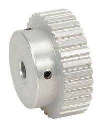
SureMotion timing pulley, aluminum, 1/5in XL pitch, 32 tooth, 2.037in pitch diameter, 5/16in bore, hub without flanges. For use with 3/8in wide belt.
