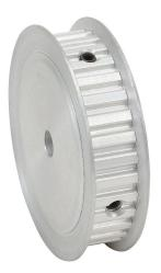
SureMotion timing pulley, aluminum, 1/5in XL pitch, 32 tooth, 2.037in pitch diameter, 1/4in bore, no hub with flanges. For use with 3/8in wide belt.
