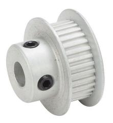
SureMotion timing pulley, aluminum, 0.08in MXL pitch, 32 tooth, 0.815in pitch diameter, 1/4in bore, hub with flanges. For use with 1/4in wide belt.
