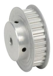
SureMotion timing pulley, aluminum, 1/5in XL pitch, 30 tooth, 1.91in pitch diameter, 1/4in bore, hub with flanges. For use with 3/8in wide belt.
