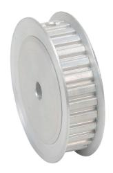
SureMotion timing pulley, aluminum, 1/5in XL pitch, 30 tooth, 1.91in pitch diameter, 1/4in bore, no hub with flanges. For use with 3/8in wide belt.
